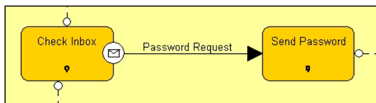
Figure 3. A message event is triggered at the end of the Check Inbox process, sending the Password Request message to the Send Password process.
